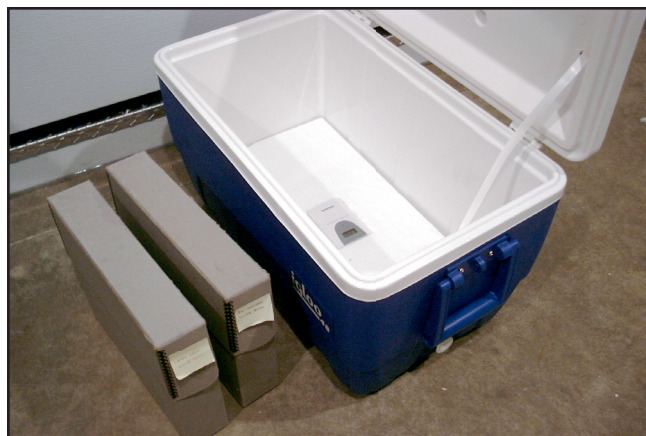
Figure 4. A transfer box for acclimatization made from an inexpensive picnic cooler. Two layers of Styrofoam (2 inch total thickness) were added to the bottom (picnic coolers typically do not have insulation on the bottom). The top layer is fitted with a wireless thermocouple (available at Radio Shack, Inc. for under $60.00). The acclimatization is complete when the thermocouple reads within a few degrees of the surrounding environment.
