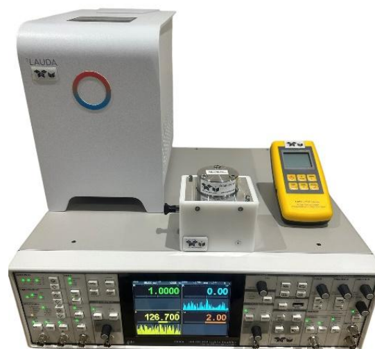
Figure 1. TriPAV equipment with lock-in amplifier, thermostat circulator, digital thermometer.
