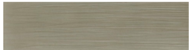
Figure 2: Example of wood grain effect. The printed image should be of uniform color.
