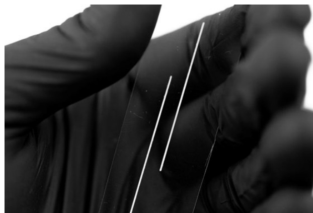
Figure 8: Lines of Elantas_45% printed with the NovoJet printhead by Quantica GmbH in Berlin
