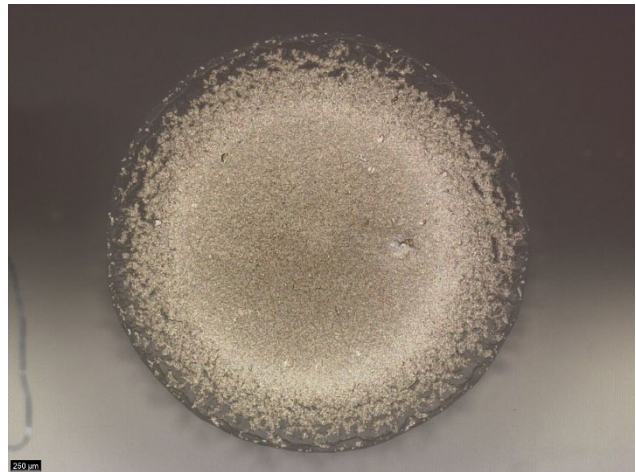
Figure 3: Droplet of Elantas_45% on PMMA substrate applied directly after mixing the solution
