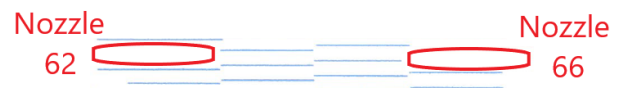
Figure 9. Visual confirmation of jetting failure. The highlighted regions show missing lines corresponding to nozzles 62 and 66, which correlate with the unstable electrical traces.
