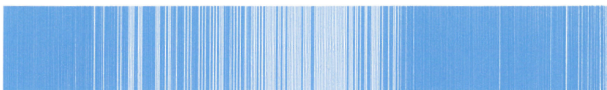
Figure 5. Nozzle check pattern. The missing print lines correspond directly to the nozzles identified as "No Load" failures in the electrical test.
