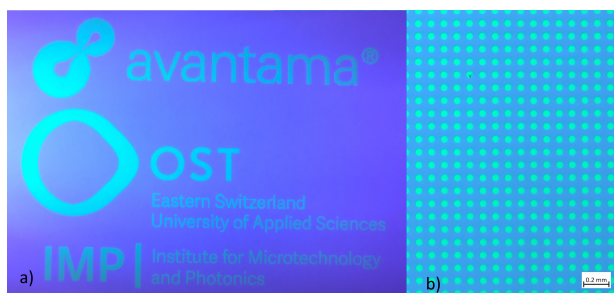
Figure 7. Paper printout of PQD ink. a) shows a photograph printed PQD logos, b) shows a microscope image of a printed dot array.
