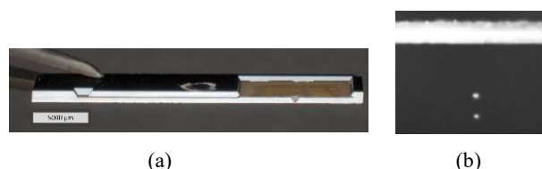
Figure 3: (a) Longitudinal section through a MEMS-based piezoelectric actuated printhead (1 x w x h: 30 x 10 x 1 mm) with the ink path towards the nozzle opening and the silicon membrane visible, and (b) two single droplets ejected by piezoelectric actuation.
