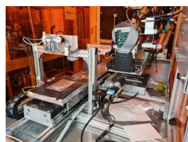
Figure 2: Inkjet printing platform
